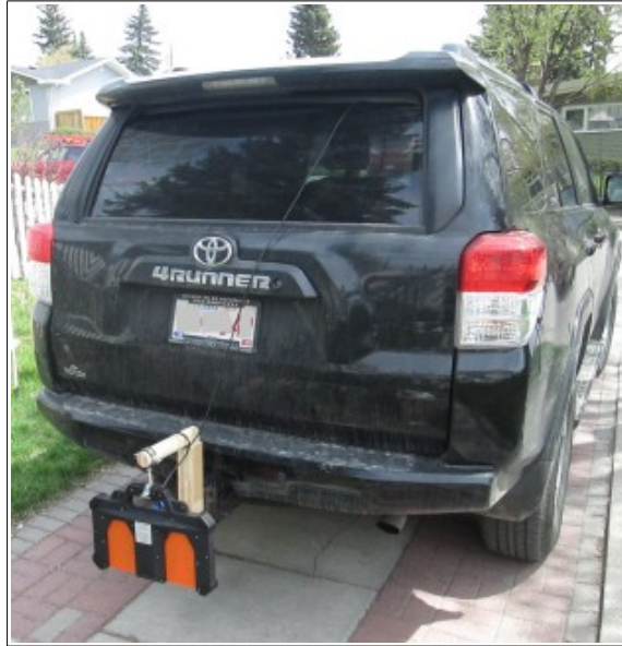
Figure 2: PicoR-Ice antenna mounting installed with the antenna module.
