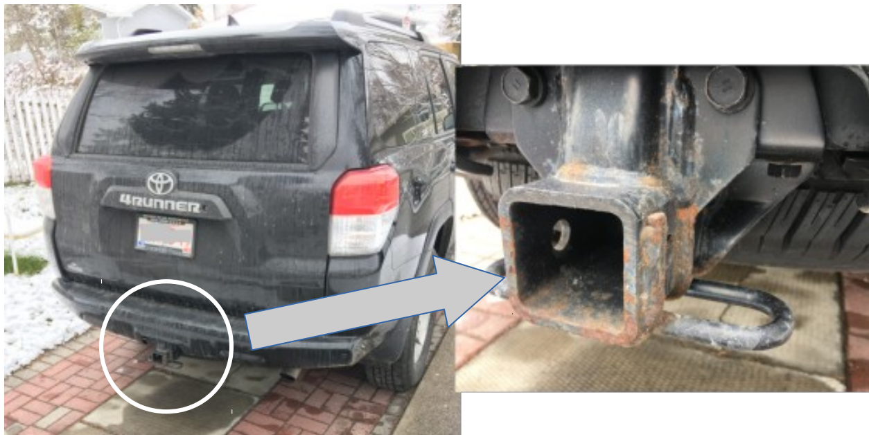
Figure 1: Location of auto manufacturer's trailer hitch (left) and detail (right).
