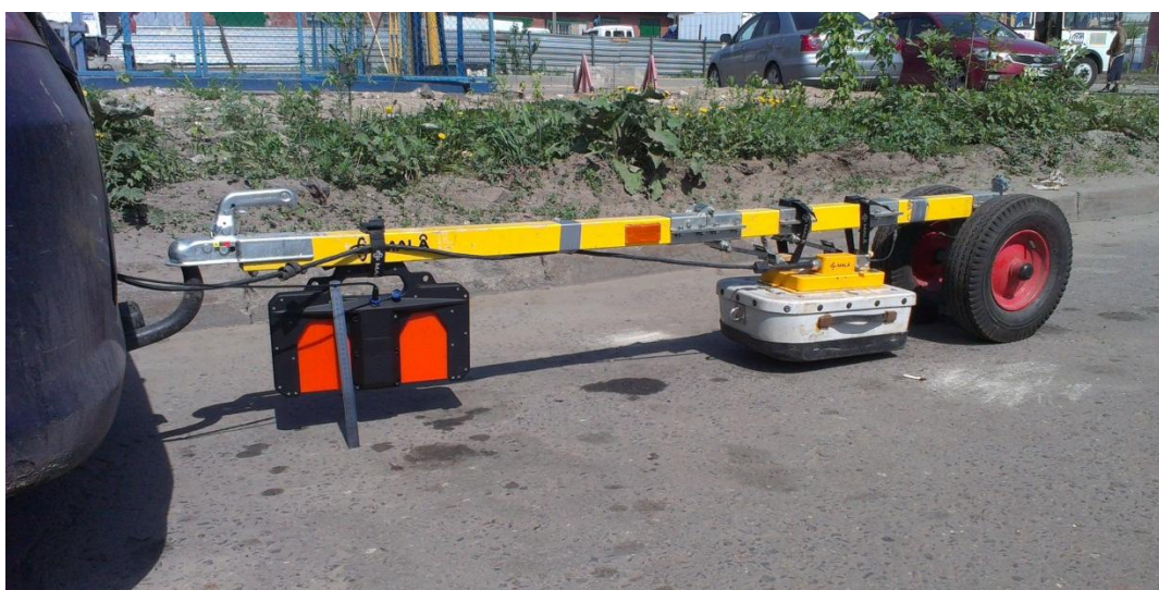
Fig. 3. Mounting the prototype module PicoR-2 in the new housing on the barbell-trailer with simultaneous mounting the antenna unit GPR ProEx 500 MHz
