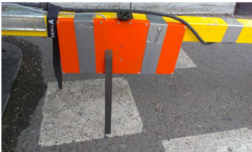
Fig. 2. Mounting the antenna module PicoR AM1 on barbell-trailer.
