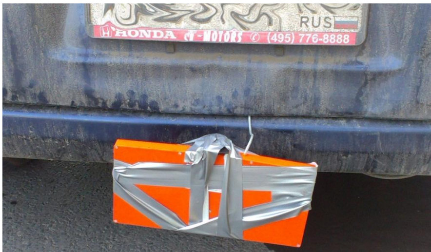
Fig. 1. Mounting the antenna module PicoR AM1 on tow bar.
